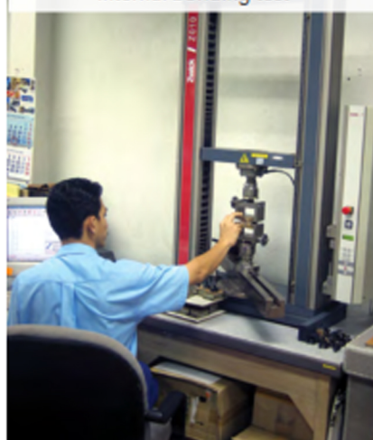
Internal bonding test
