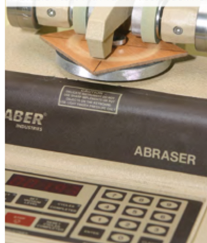
Abrasion test with Taber Test machine
