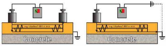
The conductive fillers are in permanent continuous contact and so there are many paths across & through the conductive system - the surface is suitable for noint to
